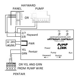
Be sure to power down your control box before doing any wiring. Using this device assumes the installer has basic electronic wiring skills.
